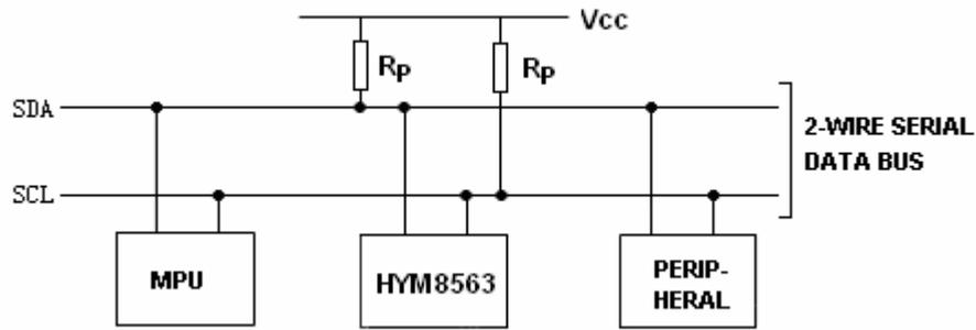
**Figure 7. Typical I<sup>2</sup>C-Bus Configuration**
