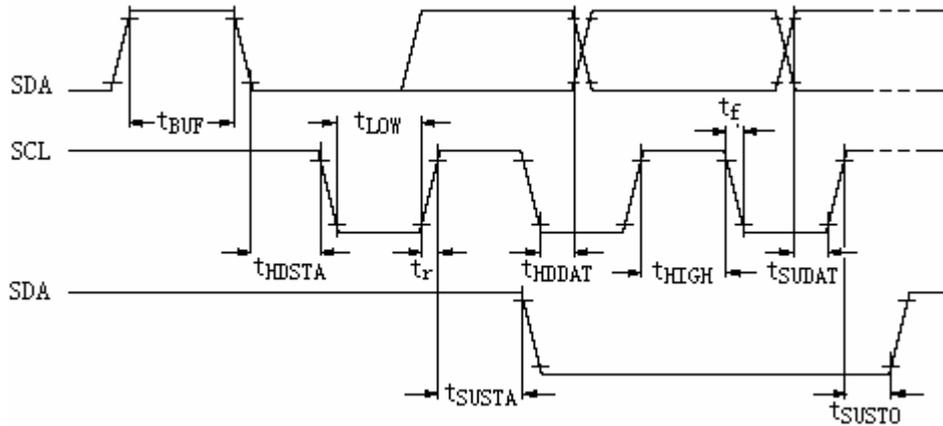
**Figure1: I<sup>2</sup>C-bus timing waveform**
