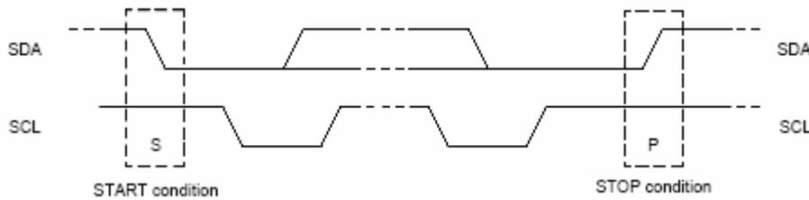
**Figure 8. Definition of Start and Stop Condition**
